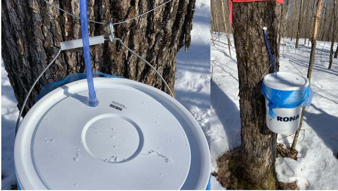
Figure 2. Experimental set-up of sap collection. Plastic tubing led from a spile into a 10 kg bucket where sap was collected in a bag to ensure independent analysis of samples. Bags were changed between collections.
