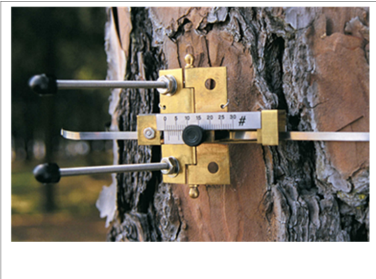
Figure 2: example of an installed band dendrometer
