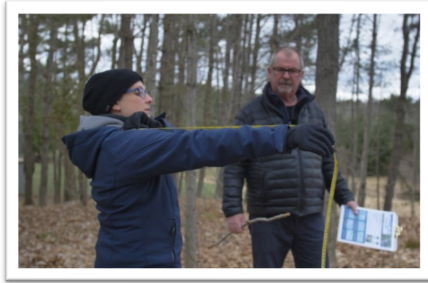
Image 7: FOTMW staff member measuring arm length as a part of the procedure to measure tree height.
