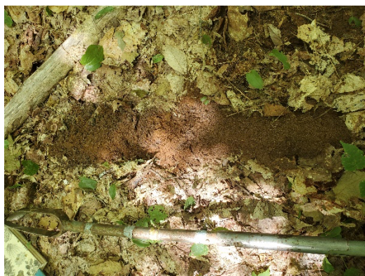
Figure 2 Site photograph of mineral horizon soil obtained using a Dutch auger, at Brookland farms.
